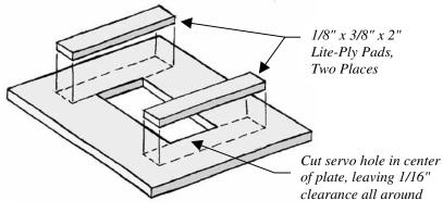
STEP 3 - Glue the assembled mounts into the wing as shown in the diagram. The mounts should be flush with the bottom surface of the wing. Glue them firmly to the ribs and spars. The lite-ply pads should face up, towards the top of the wing. You must also make a small cutout in the top wing sheeting of each wing panel for the servo wires to pass through.
