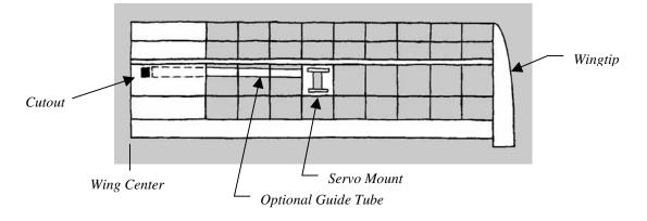
STEP 4 - Bolt your servos to the mounts using the hardware supplied with your servos. Imbed 1/16" plywood pads in the ailerons to serve as hardpoints for the nylon control horns. Use the threaded rods and clevises supplied in the Venture 60 kit for pushrods.
