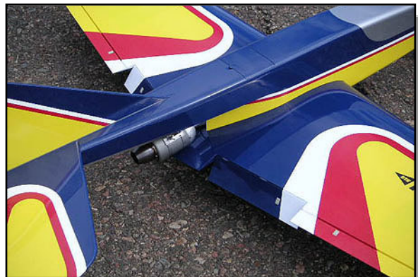
Flaps were added primarily for drag. These flaps drop about 60 degrees and provide a substantial braking effect. This photo also shows the small rear hatch on top of the fuselage for access to the manual fuel shutoff valve and fuel filling line.
