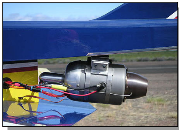
The engine thrust angle shown here was finally determined through testing. Looks funky, but it works! Notice how the front of the engine is protected from foreign object damage (FOD) from below by the trailing edge of the wing.
