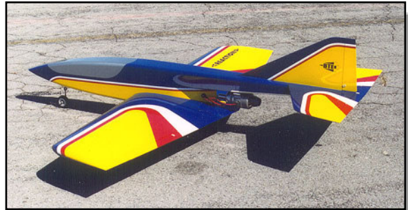
Reaction 54 in its original configuration without flaps, and engine aligned with fuselage top.
